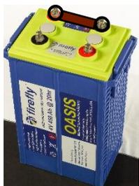
The battery will be shipped with the connection bar shown on the left. This connects the 2 cells inside the module in series making the battery 4V and 450Ah. For a 12V x 450Ah bank, connect 3 x 4V/450Ah in series (3S). For 24V x 450Ah, connect 6 in series (6S). For 900Ah x 12V, it can be either 2P (P = in parallel) x 3S, or 3S x 2P. For 900Ah x 24V, it can be either 2P x 6S, or 6S x 2P
