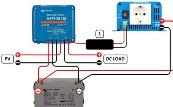
**Figure 5:** For the Victron inverters model Phoenix 12/180, 24/180, 12/350, 24/350, the Phoenix Inverter C models and the MultiPlus C models an interface cable (1) is needed: the **Inverting remote on-off cable** (article number ASS030550100)
