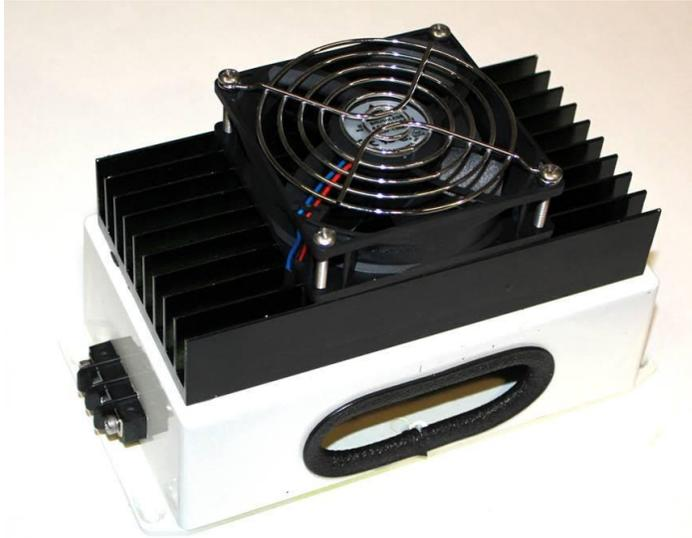
The fan is driven by the output of the alternator so as soon as current is flowing from the alternator the fan is running. As a safety backup there is a thermal switch mated to the heat sink which opens if the heat sink temperature exceeds 260degF. This temperature was chosen simply because a full current alternator mounted to an engine will run this hot but testing shows this could be lowered some, maybe 200degF in the future.
