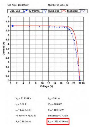
**Brand X 115w.** Note low Shunt Resistance (R<sub>sh</sub>) figure, suggesting the existence of damaged or flawed cells.
