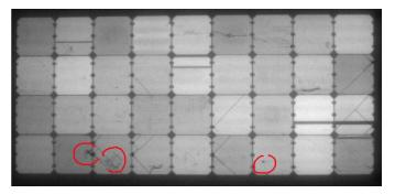
**Brand X 115w.** Note additional cracks after bending.
