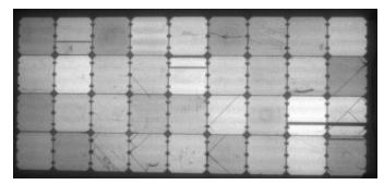
**Brand X 115w.** Cells have cracks, dings, or dark areas, indicating the existence of flawed or damaged cells.
