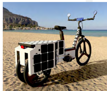
FIG. 11 The solar-assisted bicycle (which has three wheels) from IFEVS (www.ifevs.com)
