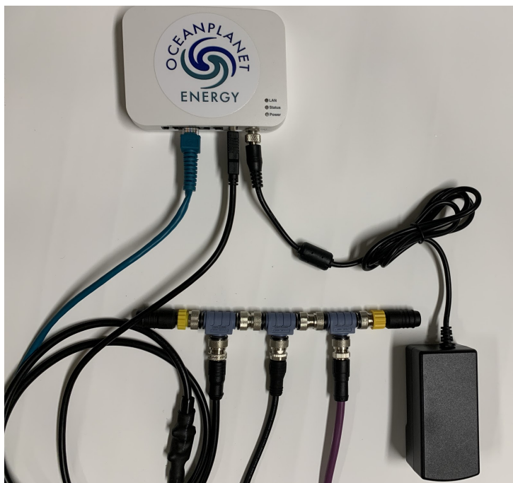
Figure 2: CAN connections shown from Left to Right. 1. CAN to tether USB port, Black cable ( sold By OPE) 2. Battery BMS connected, black cable 3. Regulator to WS/AP500 Wire Harness, purple cable (colors hard to distinguish-tw)
