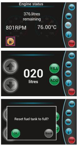
It is possible to either fill the tank with one press, or add a set amount of fuel if needed, both requiring confirmation before the fuel levels are adjusted.
