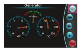
Pressing the main screen will switch between this page and a version showing the same information in text form, with more detail around the fuel usage if available.
