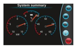
At the bottom-right is a Stop/Start button that allows you to override the system and manually turn power generation off.
