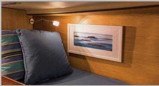
The gang at Imtra supplied me with allnew LED lighting to replace the original incandescent lights. You can see the old Pearson fitting, which is kind of cool - probably handmade by a guy in the shop but it uses a lot of power, it heats up and the lighting is just mediocre (top left). The new light is energy efficient, dimmable and rotates — just a superior product all the way around. I added another new light in the saloon that's perfect as an accent light or for reading (left).
