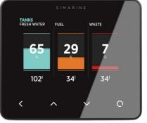
PICO can monitor up to 14 tank levels, barometric data, & can be programmed with alarms & alerts
