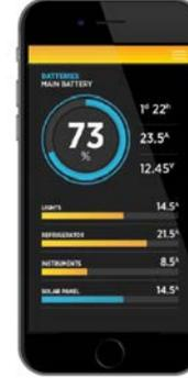
The PICO system can be monitored & programmed remotely with mobile apps for Android & I-phone
