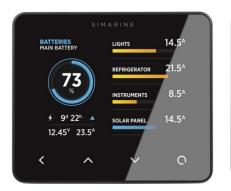
PICO provides quick view of State of Charge, time remaining, up to 20 loads, & charge sources, & much more
