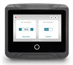
Adjust Parameters. Use the EasyView 5 to adjust frequently used settings, like the shore fuse or to switch on your inverter.
